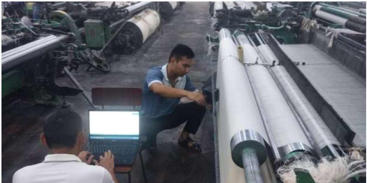
Figures 1–3. Application of the tension measuring device and the process of determining yarn tension [7]
